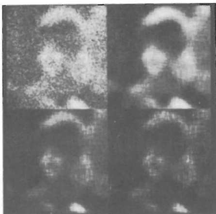
Fig. 8. Results for image 4. Image 4 (upper left), 1 step in \lambda (upper right), 4 steps (lower left), and final result after 8 steps (lower right).
