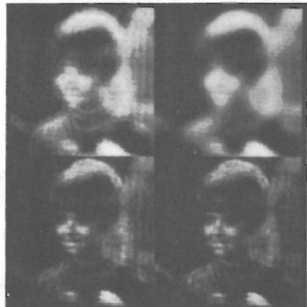
Fig. 7. Results for image 3. Image 3 (upper left), 1 step in \lambda (upper right), 6 steps (lower left), and final result after 10 steps (lower right).
