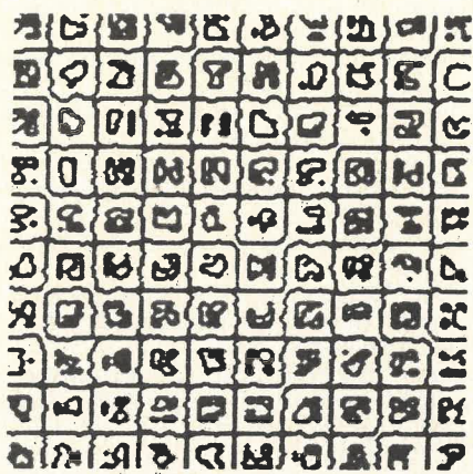
Fig. 5. The zero-crossings obtained using Haralick's implementation of the \nabla^2 G operator, for \sigma = 5.0 , limited to an 11 \times 11 support.
