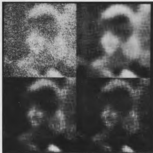
Fig. 5.4-8. Restoration results for image 4. Image 4 is shown at the upper left. The restoration is shown after 1 step in \lambda at the upper right, after 6 steps in \lambda at the lower left, and after 12 steps in \lambda at the lower right.
