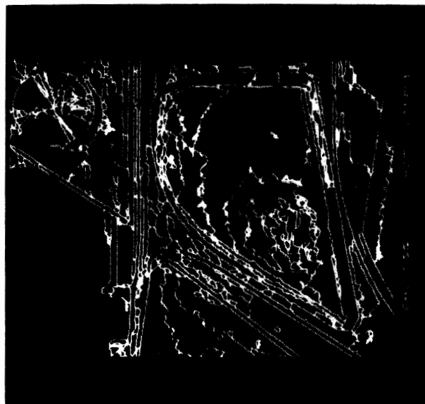
Figure B-7. Segmentation using the one-pass combined centroid and hybrid linkage method.
