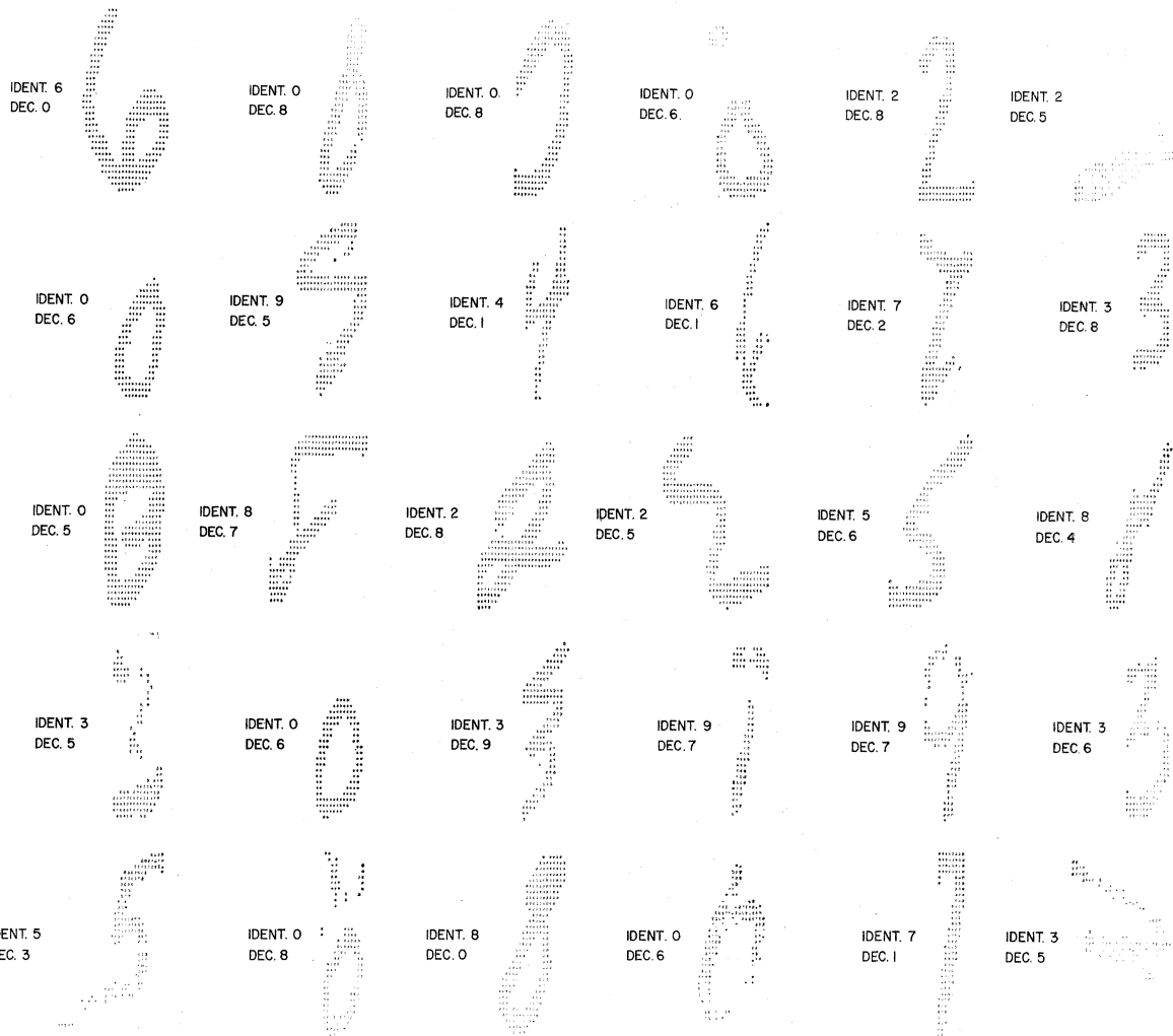
Fig. 13. Printouts of typical errors and rejects. IDENT. stands for the intended identity; DEC. for the computer decision.
