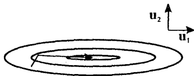
Figure 7.12. Schematic illustration of the application of the conjugate gradient algorithm to the minimization of a two-dimensional quadratic error function. The algorithm moves to the minimum of the error after two steps. This should be compared with Figures 7.4 and 7.7.
