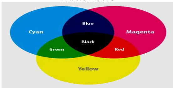
Figure 8: CMY (K) subtractive color model representation [5].
