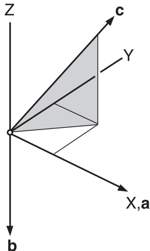
Base vector **a** points into X-direction, **b** into negative Z-direction and **c** is along the diagonal in XYZ.
